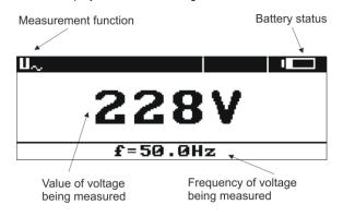
Fig. 12 Alternating voltage measurement - result
