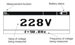
Fig. 2 Screen layout in alternating voltage measurement mode
