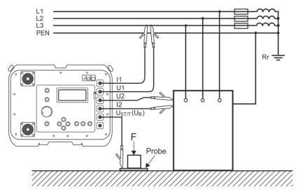
Fig. 15 Measurement of shock voltage U<sub>T</sub>
