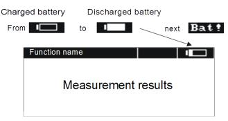
Fig. 34 Battery charge indicator
