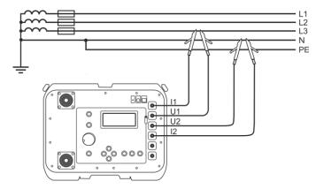
Fig. 21 Measurement of impedance in working circuit (L-N) using four-pole method
