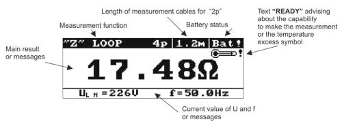
Fig. 4 Screen layout in short-circuit loop impedance measurement mode (main result only)
