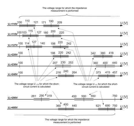
Fig. 13 Relationship between the network voltage and the ability to calculate the short-ciruit current
