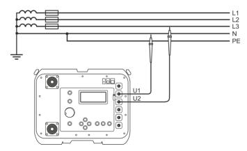
Fig. 11 Alternating voltage measurement
