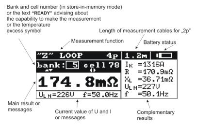
Fig. 3 Screen layout in short-circuit loop impedance measurement mode (all results)
