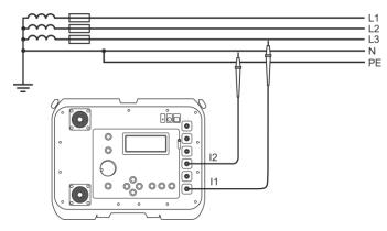
Fig. 17 Measurement of impedance in working circuit (L-N) using two-pole method
