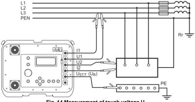
Fig. 14 Measurement of touch voltage U<sub>ST</sub>
